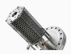
The CapaciTorr® D 2000 pump is based on high performance SAES® St 172 sintered porous getter disks. The getter cartridge is provided separately from the CF100 or CF150 base flange, which incorporates a built-in heater that directly connects to the flange power feedthrough.
