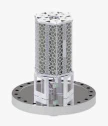
The CapaciTorr® Z 2000 pump is based on high performance SAES® ZAO® sintered porous getter disks. The getter cartridge is provided separately from the CF100 or CF150 base flange, which incorporate a built-in heater that directly connects to the flange power feedthrough.
