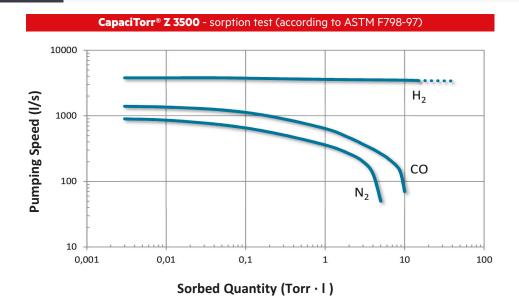
**Typical Pump Characteristics** CapaciTorr Z 3500 ZAO Alloy Type Zr V Ti Al Alloy Composition Getter Mass (g) 705 Getter Surface (cm<sup>2</sup>) 3900 Activation Power (W) 360  $H_2$ 3900  $H_2O$ 2100 Pumping Speed (I/s)  $N_2$ 900 CO 1400  $H_2$ 14100  $H_2O$ >200 Sorption Capacity (Torr•I)  $N_2$ 5.1 CO 10
