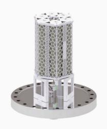
The CapaciTorr® Z 3500 pump is based on high performance SAES® ZAO® sintered porous getter disks. The getter cartridge is provided separately from the CF150 or CF200 base flange, which incorporate a built-in heater that directly connects to the flange power feedthrough.
