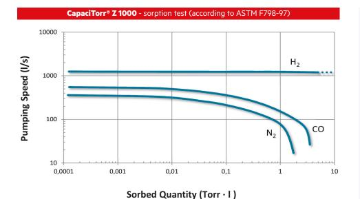
**Typical Pump Characteristics** CapaciTorr Z 1000 ZAO Alloy Type Zr V Ti Al Alloy Composition Getter Mass (g) 280 Getter Surface (cm<sup>2</sup>) 1530 Activation Power (W) 190  $H_2$ 1250  $H_2O$ 900 Pumping Speed (I/s)  $N_2$ 360 CO 550  $H_2$ 5600  $H_2O$ 70 Sorption Capacity (Torr•I)  $N_2$ 1.7 CO 3.5
