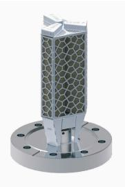
The CapaciTorr® Z 1000 pump is based on high performance SAES® ZAO® sintered porous getter disks. The getter cartridge is provided separately from the CF63 or CF100 base flange, which incorporate a built-in heater that directly connects to the flange power feedthrough.
